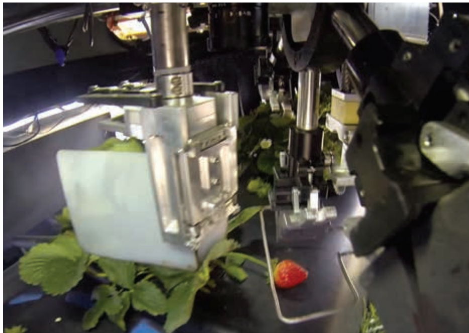
Harvest CROO Robotics, Tampa, FL, has developed a strawberry picking robot that crawls through the fields and harvests fruit based on an advanced vision system.
